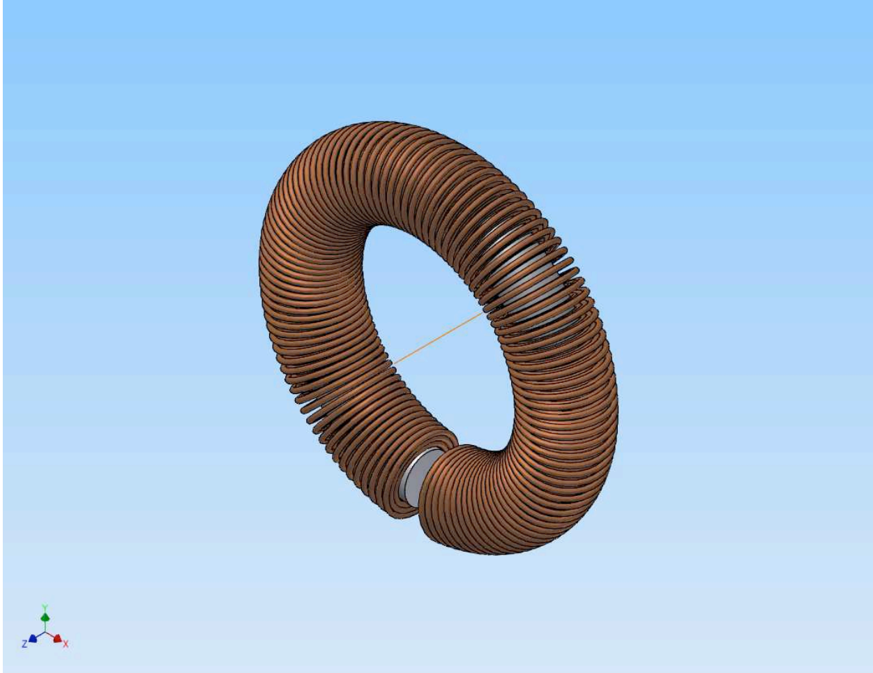
Figure 2. Typical “C” Core magnet (shown with metal core)
