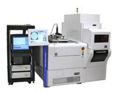
SANTA CLARA, CA – Sep 25, 2015: Integral Solutions International, ISI, the world's leading manufacturer of Quasi-Static testers for the data storage industry, announced today the release of 5,000 Oe Perpendicular Magnet for the ISI WLA-3000 Wafer Level Analyzer for STT-MRAM characterization.
