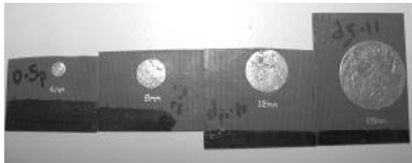
Figure 1b. Four disk capacitors 0.5pF, 2.2pF, 4.4pF and 11.5pF.
